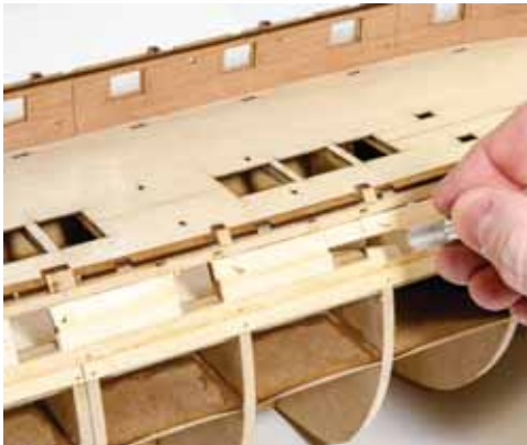
153. When the planks are dry, remove the pear bulwark sections and then use a razor saw to roughly open-up the gun ports. These will be trimmed closer a little later.
