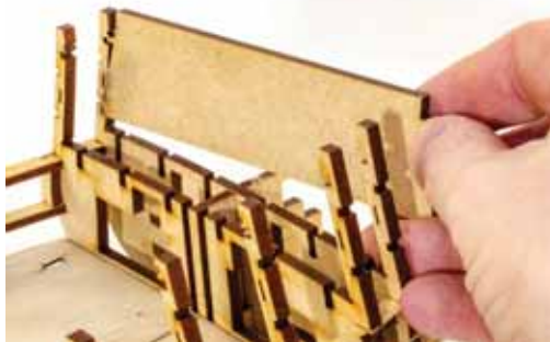
99. Carefully remove the plank panel from bulkhead #18. You can do this by gently twisting at the part and pushing in either direction while supporting the bulkhead ears. That panel can now be discarded.
