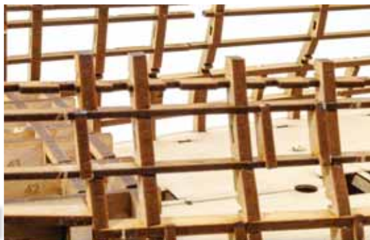
123. Now glue into place as shown here, with #52 being the foremost vertical gun port strip (adjacent and aft of bulkhead #15), #53 being the other side of that port, slightly aft, and #54 fitting into the frame notches in the area that you cut away part of bulkhead #18.
