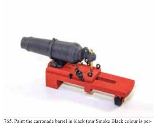
765. Paint the carronade barrel in black (our Smoke Black colour is perfect for this), and glue to the gun to the base. Take a length of 0.7mm brass rod and glue as shown. You may need to very slightly open up the gun hole at the rear. Paint the rod black.
