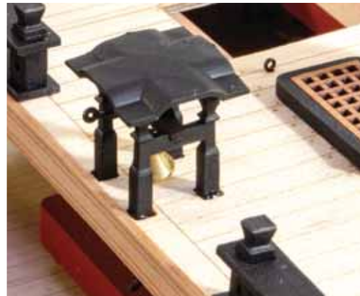
802. Glue the completed belfry into position. You can use a short length of 0.25mm rope to dangle from the end of the belfry (not shown here).
