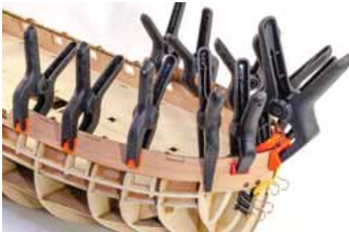
146. Clamp these into place on the hull (DO NOT GLUE). You may find it necessary to soak these parts for 30 minutes in warm water. If you do this, you MUST leave the parts for 24hrs to dry and to shrink to normal size again as pear expands a lot when wet. Note that the main bottom edge of this part lies along the top of the fore gun port frames.
