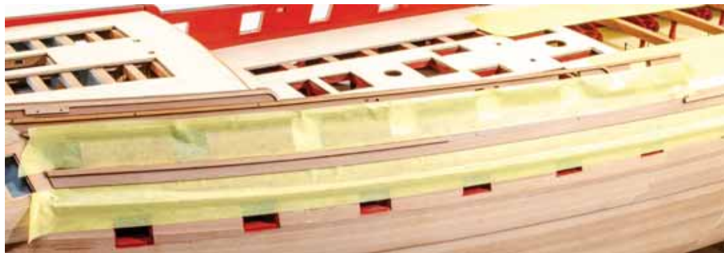
528. Take a 2mm x 1mm strip and glue along the top edge of this section of the strips you just added. Stop that strip where the rearmost channel position is that you marked earlier.
