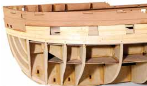
162. The plank can now be glued and pinned into place. All planks must be glued to each other as well as to the bulkheads.
