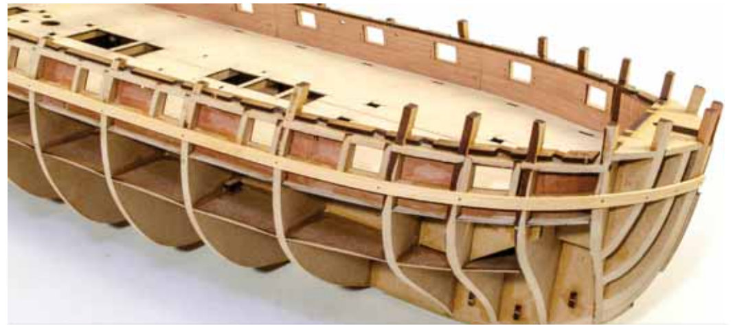
148. You can now remove both of those parts until later. As for now, planking begins. Take one of the 1.5mm lime strips and run it from the bow through to the fore bulkhead #9. This first plank will run along the bottom of the gun port frames. For forming the planks around the bow, we highly recommend using a plank nipper to help form the curve. These are available in our web store.
