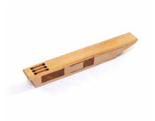
594. Now glue the top and bottom parts #424 and #425 into place and clamp until dry.
