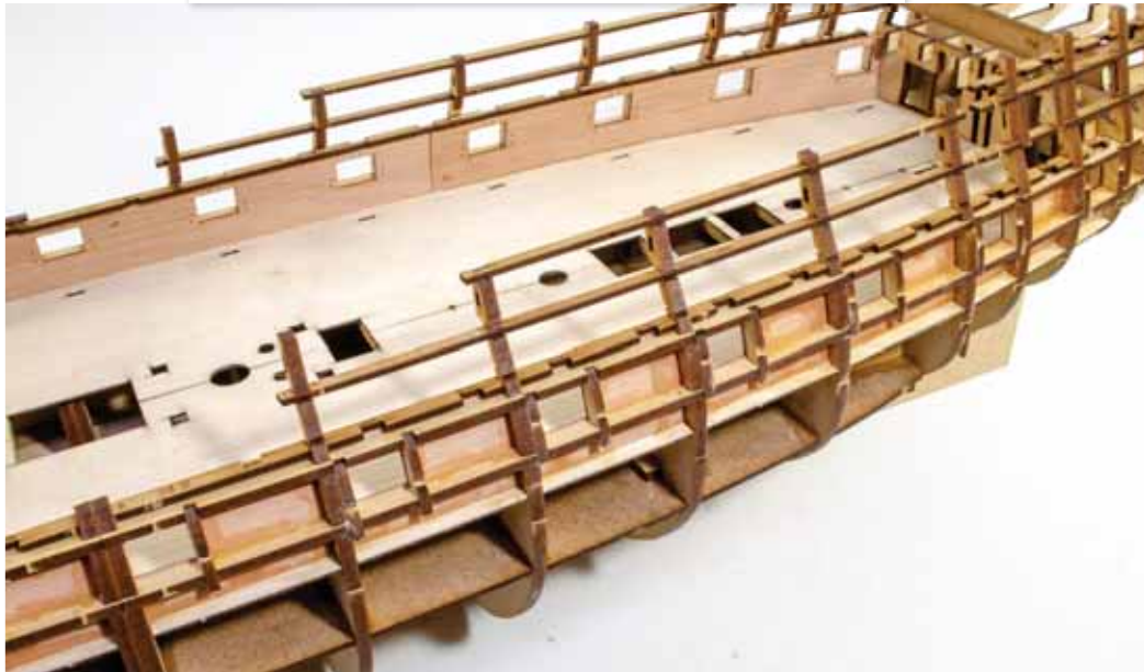
138. Fit (NO GLUE!) these strips into the bulk ear slots running from bulkhead #9 thru to #16.
