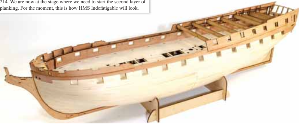
215. Using the pear planks F-62, we will now start to add the second layer. Glue your first and second planks, one after the other, directly underneath the outer pear bulwarks that you added.
