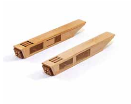
595. Glue part #430 onto the square end of the cathead and then the smaller #431 onto that.
