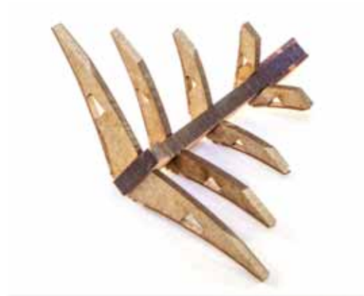
605. Use a sanding stick to level the tops of the frames between the largest and second largest. Then add a level between the second largest and the next in line. These are where the bow grates will sit, and the grates need as much of a connection as possible when seated on these frames. Now sit the assembly to one side.
