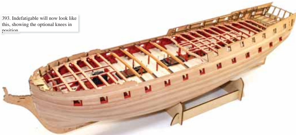
392. OPTIONAL KNEES: The beams you just installed also have optional knees. If you feel comfortable adding these, or consider it worthwhile, then you'll find the information you need on your plans. Remember, the longer side of these is the face that sits under the beam, while the shorter side will sit against the inner bulwark.
