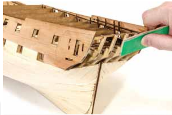
166. The back edges of the bulwarks are now trimmed to match the shape of the stern frames.
