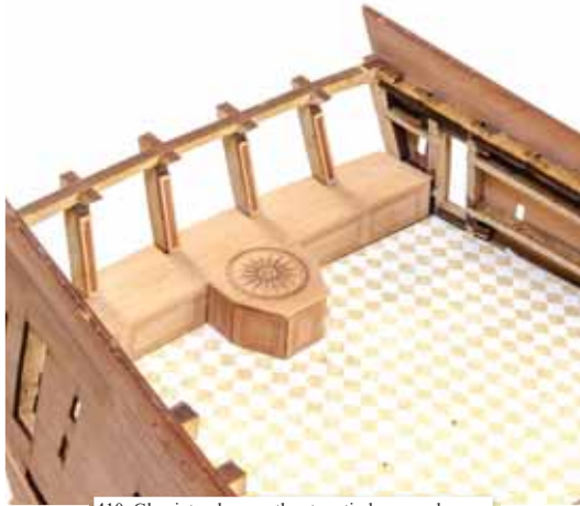
410. Glue into place on the stern timbers, as shown.
