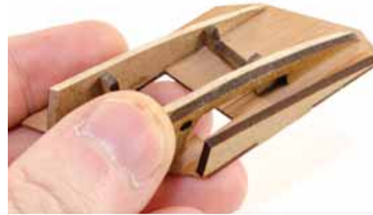
190. Glue this to the bottom slot on the quarter gallery assembly so that it's spaced evenly all along, in relation to the part you just glued into place. Leave to dry.
