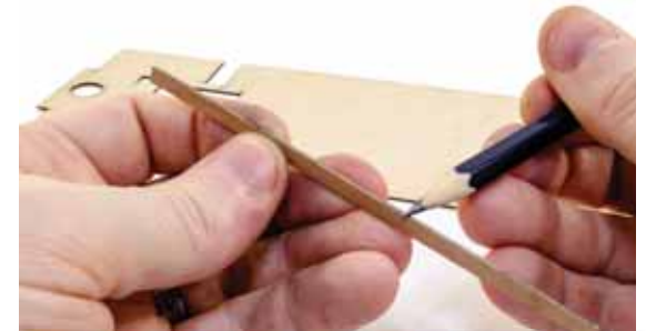
(b) Use a soft pencil to colour the edges and ends of each strip. This will simulate caulking.
