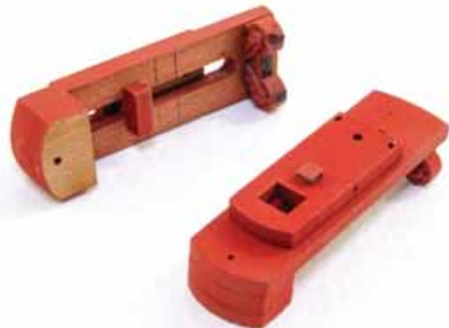
445. Sit (DON'T GLUE) part #154 on top of #153, and then insert/glue part #158 through the base and into the sliding bed #154. Leave until dry and make sure the part slides easily enough.
