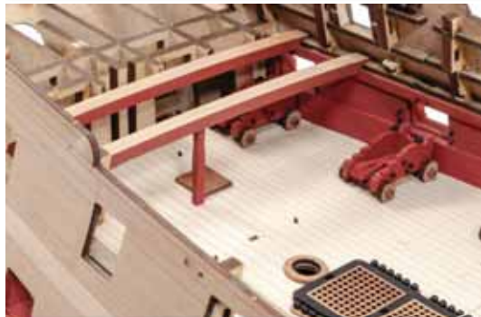
361. Here you see the second deck beam installed and supported on a painted pillar. As this is directly to the deck, the pillar is a DPL. These are clearly indicated on the plans.
