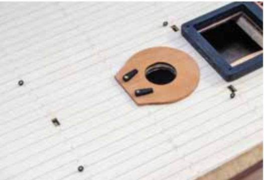
311. Paint both parts #283 (pawls) and use brass pin to locate them. Don't glue just yet.
