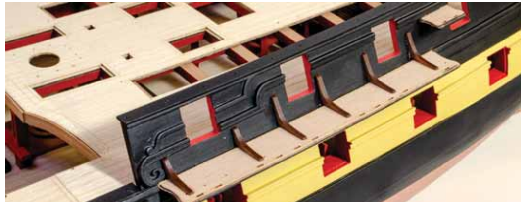
667. Now glue the channel knees to the channels, referencing your plans for the correct knees. Whilst the angles of the knees should be very close (if not correct) to your hull, you will need to profile them differently against the hull as you move forward along the fore channel. This is where the hull angle will change from station to station.
