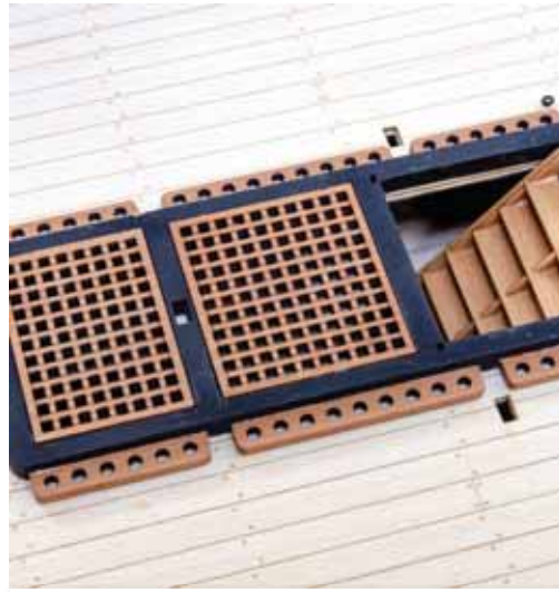
272. From the 1.5mm wood sheet, remove parts #189 and #190 and glue into place as shown here.
