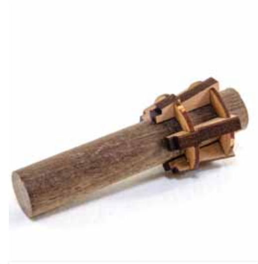
314. You can verify that everything is correct by inserting the dowel through the assembly (DO NOT GLUE). You can leave this part in place for the next stage.
