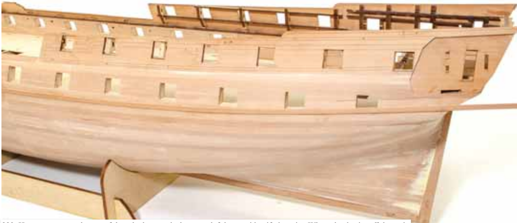
223. Here you can see the run of that plank towards the stern, left long to identify it easier. When glued, trim off the end.
