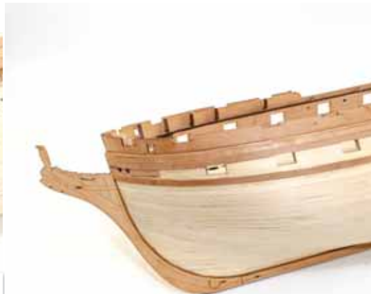
217. Now add another pear strip along the underside of those marks. The front of this plank will lie in line with the top of the prow. This plank will mark the position of the upper wale plank you will later add, so this is why the position of this plank is important.
