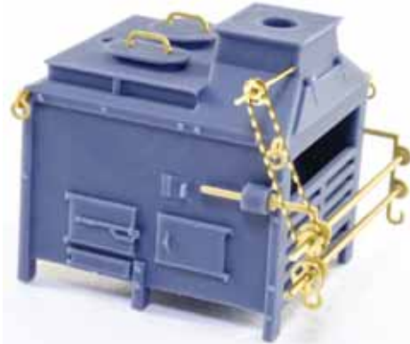
344. Slide the shorter chain BS-7 between the thin upper brass rod and the thick top brass rod. The chain link detail will face outwards. Now push this and the previous brass parts towards the stove body so they don't foul any other stove area. Add a spot of CA to fix.
