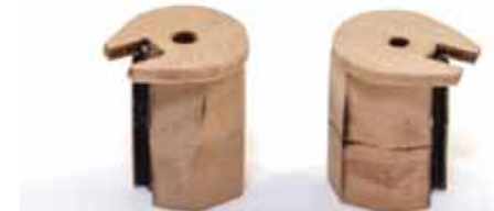
328. Glue part #442 to the top of this, making sure the hole is central to the hole in the wooden assembly, and that the slot aligns.
