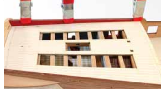
498. Paint these parts in red and fit to the inner bulwarks on the poop deck.
