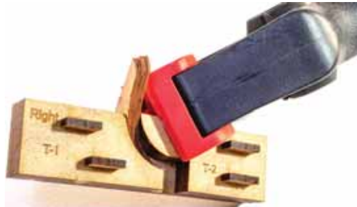
620. Soak these pieces in hot water for 30 minutes, then sandwich them together (no glue) and position in the jig as shown, closing up the sliding side to induce a curve in the parts.
