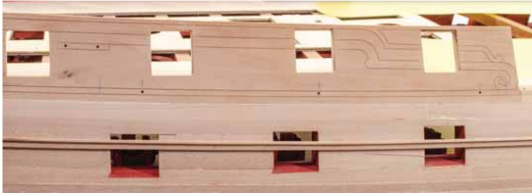
516. Notice the engraved marks on the upper, outer bulwark. These denote the position for the front and end of the main mast channel, and the holes for pinning it in place. Transpose those marks, using a pencil, so they are marked just above their positions.
