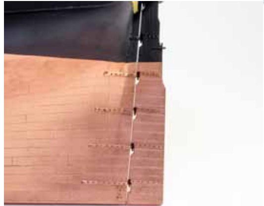
589. The rudder can now be finally glued into place. You should now fit the rudder straps to the hull, R-1 to R-6 and copper them in the same manner. You may also find it useful at this stage to protect the copper using a sealant or varnish etc.
