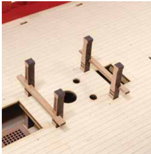
251. Push all parts #88 into their holes as shown (DO NOT GLUE), and then glue parts #126 across them. Leave to dry and then carefully remove the assemblies and set them to one side.
