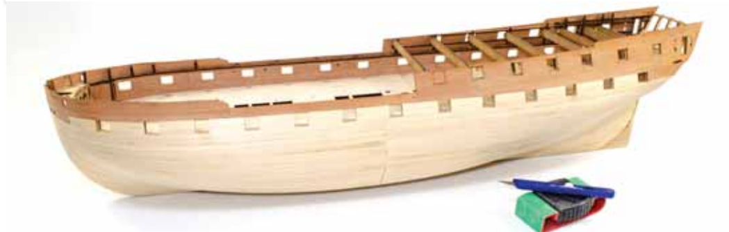
164. Sand the hull. This is a large and heavy hull, so we suggest using an electric palm sander to help with this task. You will also create a lot of dust, so don't forget to wear a mask. At this point, I also clean up the gun ports, so they are more or less the same size as the framing.
