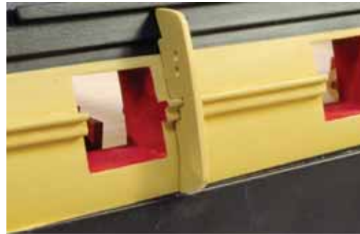
651. Locate the position of these from the plans and notch the parts to suit the position of the rails on your hull. Paint the parts yellow and glue to the hull.
