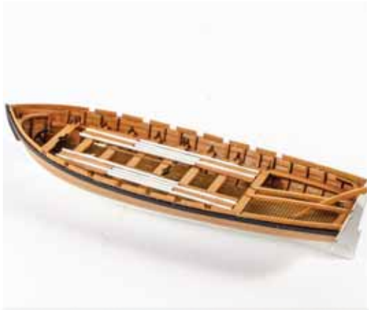
917. Fit the oars as well as the boat hooks and anchor. You can also see that we have photos of the boat with the rudder stowed.
