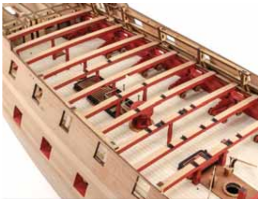
363. Here we see all the quarterdeck beams installed. Well, almost...
