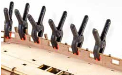
130. We suggest that you initially clamp the parts into place after multiple test-fits and any trimming (if needed). Remember that the port holes in these will be slightly smaller than the frames, to allow you to trim those areas later. Once you have clamped these in place, glue can be painted into the joints from the rear. NOTE: As wood is a natural product, some wood can be stiffer than normal. If you find this with yours, soak the parts in hot water for 30 minutes and when clamp into position until dry. We suggest no less than 24hrs to allow the part to return to its pre-soak size, before gluing.
