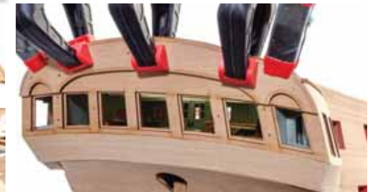
482. Carefully glue into position on the stern, using the engraved lines to guide you.
