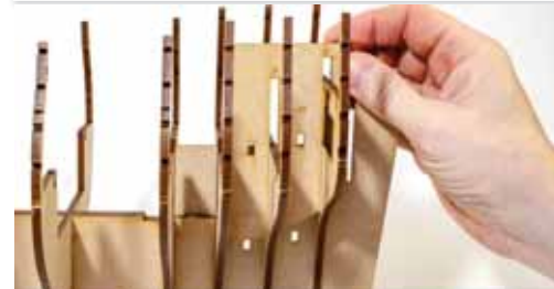
21. As with the previous parts, slot one of these on either side of the keel, holding bulkheads #15 and #16 into position. Bulkhead #17 is only there at the moment to ensure correct positioning of the current parts.
