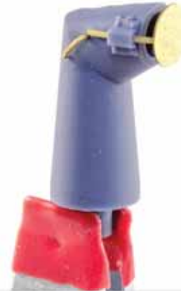
349. Take the stove chimney and add two small handles BS-2, and also the plate which obscures the opening, BS-9. This will need to be bent to shape and fitted so there is a millimetre or so clearance between the two.
