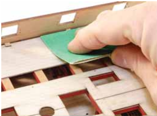
400. Make sure you use sandpaper to totally level any MDF which may still remain above deck height.
