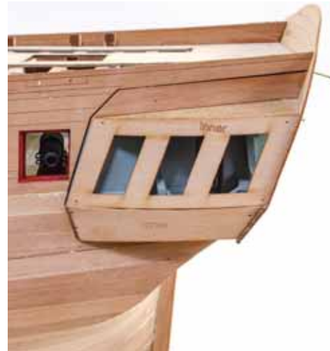
468. Now fit the lower part #568, bevelling the top edge so it sits up the previous part. You will need to trim this part to suit your own specific build.
