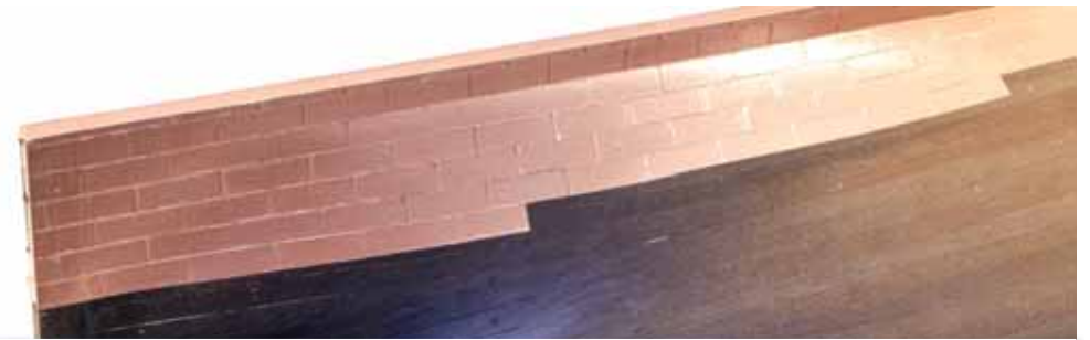
570. One of the spare lengths of copper tape was first added as a full strip along the top of the keel, where it meets the hull. The plates were then scored into this with a knife, using a cut copper plate as a template. NOTE: It's important that you keep the tape as straight as possible when you peel the backing off. To do this, we suggest that the end you peel is fastened to the knife blade you will use, and the backing is peeled from the tape, and NOT the tape from the backing! This is important as if you just peel and pull the tape away from the paper, the copper will crease and look distressed. Keeping the tape straight and removing the backing will remove most/all of that problem. Work up from the keel with your coppering, towards the waterline. IMPORTANT: You are advised to wear latex/vinyl gloves when coppering so that the acids on your skin don't 'etch' into the delicate tape surface. Whatever you decide, it's advisable to wash the finished coppering with ethanol/isopropyl and then gently finish with 0000-grade steel wool before adding varnish to it.
