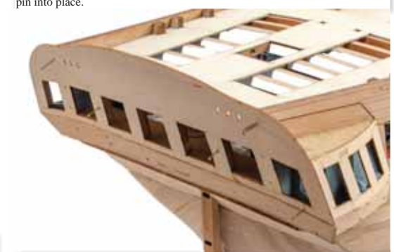
469. Here you can see the flow of the stern, from the quarter galleries to the rear. The transition in the gallery angles must match those of the stern so that the rail will eventually fit without being staggered. This is extremely important if you want your model to look correct.
