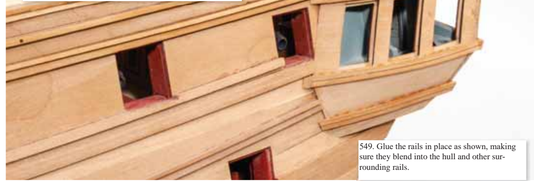
549. Glue the rails in place as shown, making sure they blend into the hull and other surrounding rails.
