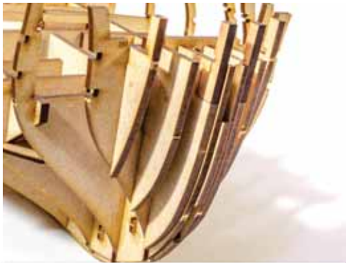
69. The assembly will look like this. Remove the bulkhead #1 assembly from the hull.
