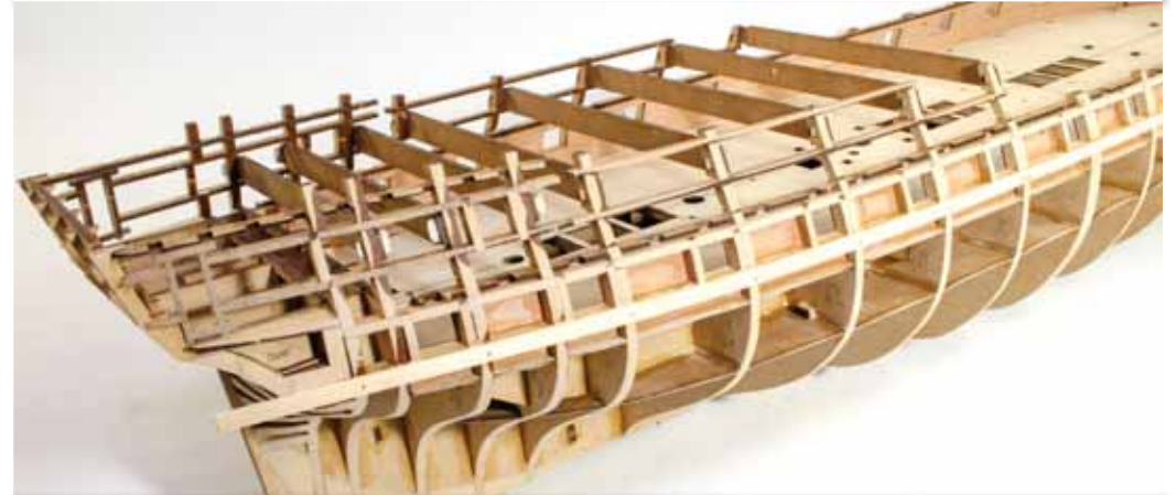
149. When you have fitted the first plank, you can continue that plank run using another strip of lime, again, continuing the run underneath the gun port frames. You can pin these planks into place until dry.
