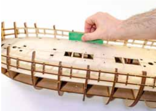
127. Before any other work can commence, you need to sand the inner bulwark frames, so they are smooth. This can be a little time consuming but doing this properly will pay off in the next stages. Just be careful with the frames at this stage.
