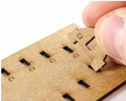
821. 18ft Cutter: Indefatigable has 4/5 boats fitted to her. Locate all the hull frame parts and jig on the 2mm MDF sheet. All of the parts are grouped together. Remove all the parts and dry fit the bulkheads into their correct base slots.
