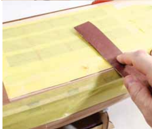
513. Mask all hull openings and sand the waist bulwarks down to flush with the waist gangways.
