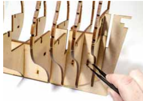
22. Glue pegs K-1 through the keel to lock bulkheads #15 and #16 permanently. You can now remove bulkhead #17 until a little later.
