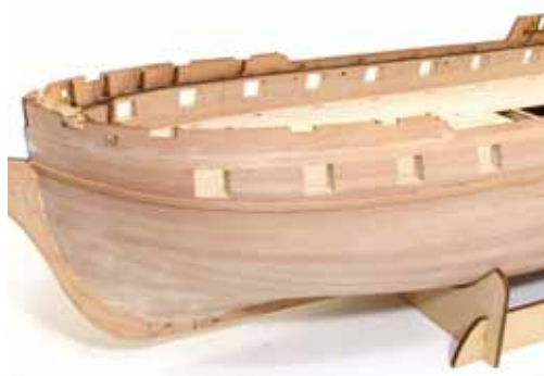
222. Glue a 4mm x 1mm pear strip F-63 to the hull, following the position of that plank you earlier added to the positions below the gun ports.
