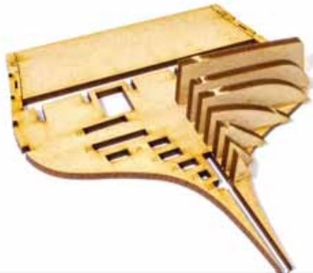
78. Glue the parts to bulkhead #18, using the slot reference numbers to help you with the correct part placement. Do this for both sides.
