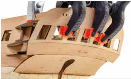
184. Cut along the pencil line you have just drawn and remove the lime planking from above the line. Now glue the inner part #402 into place, pinning it until the glue has set. Ensure the part is also central before you pin.
