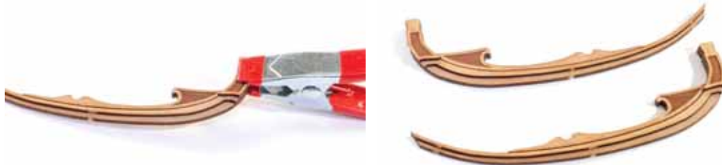
611. Now do the same for the head timbers which will install to the opposite side of the bow.
