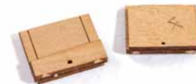
817. Some ports, such as this, also include an extra outer part which will match the wale into which the gun port is fitted. These are self-explanatory.
