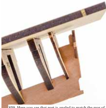
859. Here you see that part is angled to match the rear of the keel.
