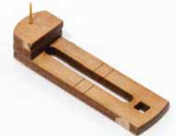
440. Glue both parts #157 on top of each other and then glue this to the engraved underside of part #153. You can use some wire to temporarily align the parts and then later remove it.
