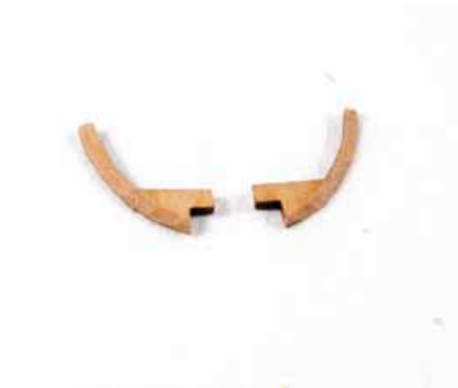
892. Take parts L15 and shape/bevel like this.
