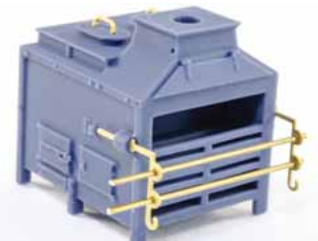
340. Cut two lengths of 0.8mm brass rod as seen here, and glue into place. You can cut these slightly overlong on the left of the stove as they can be trimmed to length after.
