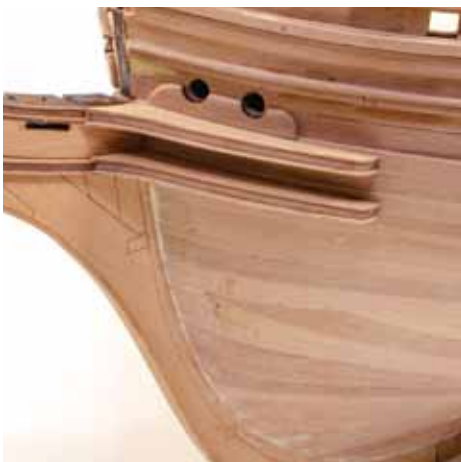
562. Sandwich the 2mm parts between the 0.6mm parts. It's an idea to round the forward edges of the 0.6mm parts first, for aesthetics.
