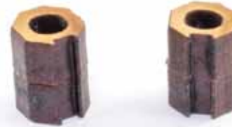
327. Take the 4mm wooden parts and glue one to another, making sure the slots align. Two assemblies are shown here.
