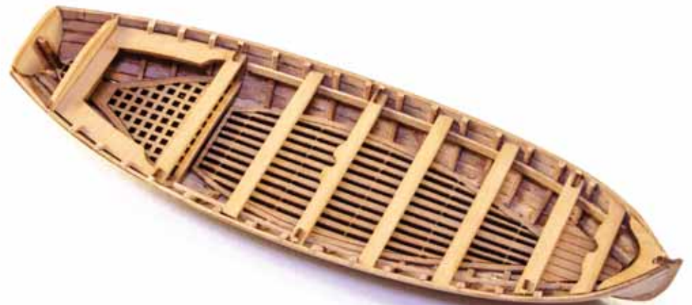
940. Fit these into the hull and fit the thwart knees.
