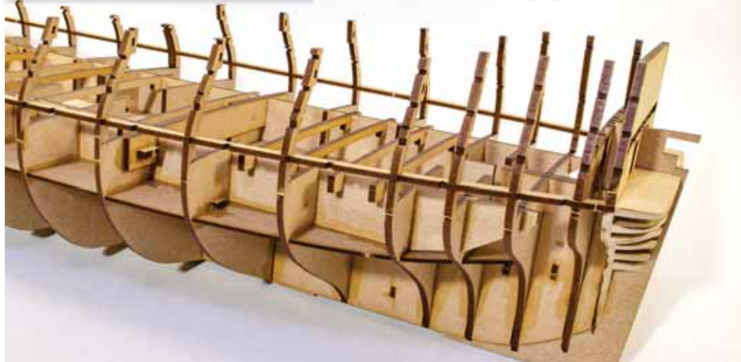
87. These are now fitted to the same extended row of bulkhead notches, extending from bulkhead #9 thru to bulkhead #18. Again, either glue these in straight away or fit them brush glue into joints.
