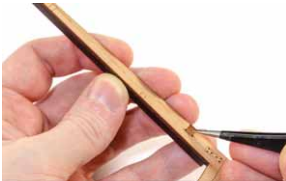
198. Glue the facings to the rudder post, one either side so the engravings face outwards, and glue in the pegs to help with alignment.
