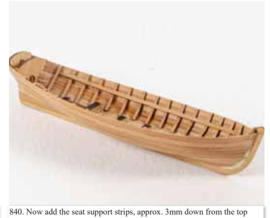
840. Now add the seat support strips, approx. 3mm down from the top edge of the bulwark.
