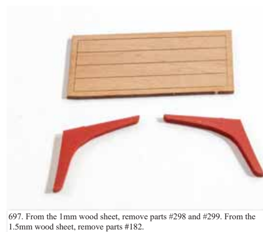
698. Paint the latter parts in red and glue to the underside of the gangway parts as shown here. You can reference the spacings on the plans.
