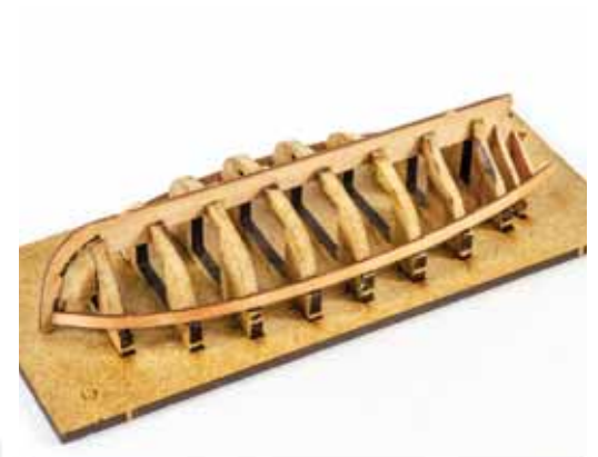
828. Glue the first planks from the 0.6mm wood sheet. These fit onto the shoulder of the jib bulkheads. Note the 0.6mm wood sheet has more part for this boat, grouped together.
