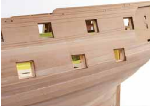
232. Here you see ports #11, #12 and #13 with their liners fitted.
