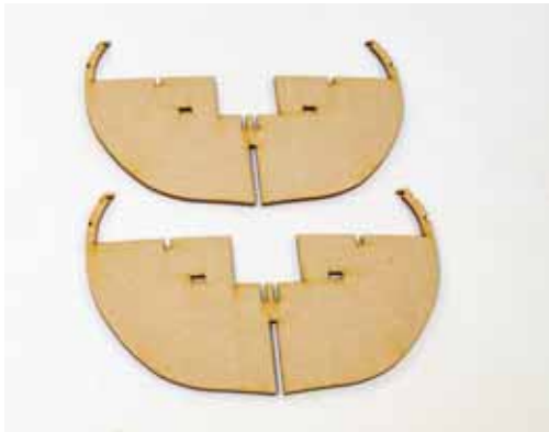
7. Also remove bulkheads #9. You'll notice there's two of these. These are both needed.
