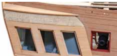
478. Glue the 3mm parts together while temporarily sitting them underneath the quarter galleries. When set, sand to profile as shown and fit to the hull. The 1mm parts need to be carefully shaped so they just overhang the roof, and the outer edge rounded off. Glue to the model.
