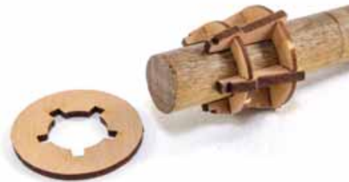
736. You can use a section of dowel to align the parts. This is only dry-fitted. From the 1.5mm wood sheet, remove part #162.
