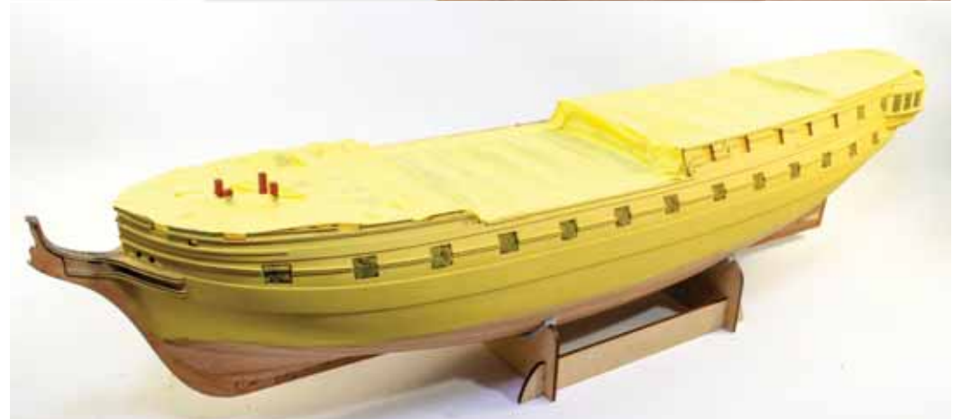
566. After carefully masking the hull and blanking any openings, paint the hull in yellow ochre. If you comprehensively mask any openings, you can airbrush this colour. Note that all of the area to be painted is now in ochre. The reason is that the lighter paint makes it easy to see any defects in the hull at this stage. Paint using thin coats, run back and fill as necessary.
