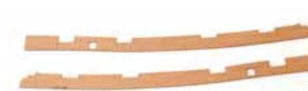
205. Remove both parts #228 from the 1mm wood sheet. These are identical but will be used on opposite sides of the bulwarks.
