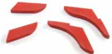
382. OPTIONAL HANGING & LODGING KNEES: There are certain things you can add to a model which generally aren't easily seen, or seen at all! One request we've had was to include the lodging and hanging knees that sit in the corners, between deck beams. Here you see the hanging knees, painted. The short ones are to fit into positions where there is a gun port directly below.
