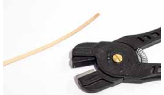
161. Again, a plank nipper is a great tool for helping form the curves in this 1.5mm lime. There's no need to soak to bend planks, and with any subsequent shrinkage that would occur.
