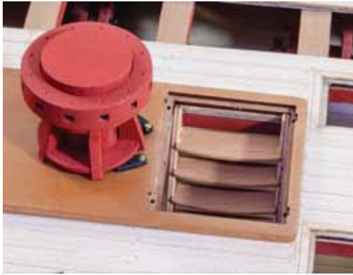
747. Glue the ladder into place as shown, followed by the capstan and also the pawls #283 from the 1mm wood sheet.
