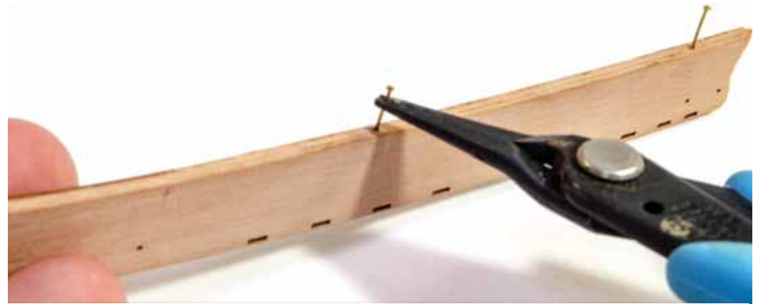
665. Test fit the channels against the full and bevel as needed to ensure a snug fit. Do not insert pins into the core. The part is laser-cut to present a place into which to push the pins. If necessary, drill slightly to open up.
