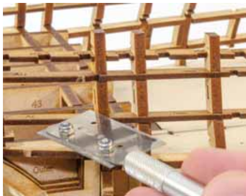
121. Carefully saw out this specific part of bulkhead #18 and file the area smooth. Also note that you can also saw and file away the parts of the strips that pass through the quarter gallery doorways.
