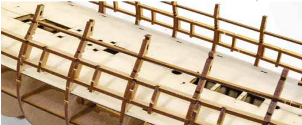
114. Now glue these into the bulkhead slots that run from bulkhead #10 thru to bulkhead #14. You do not need to glue where the part touches one of the previous 'AL' rail you recently installed. In fact, there should be a small gap at that point anyway. If not, don't worry at all about that.
