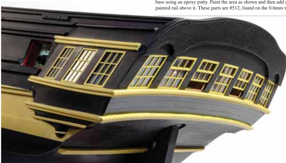
638. It's now time to consult your plans and first install the windows into the openings. These are found on the 0.5mm PETG sheet. Remember, you can install the stern windows either open or closed, or a combination of both, as seen here. Paint the window frames in ochre and install over the glazed parts. The frames can be found on the 0.4mm PE sheet. Don't get the frames mixed up as each is specific to its opening.
