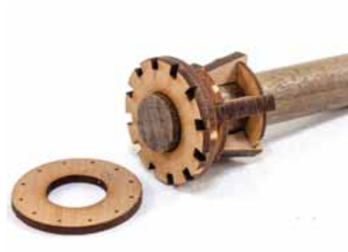
317. Glue into place on top of the previous part, as shown. Temporarily fitting the dowel can help with alignment. From the same wood sheet, remove part #160
