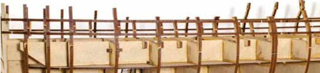
93. The first gun port is number 1, then going backwards they are number 2, 3, 4, 5, 6, etc. Glue each pair of vertical gun port strips into their respective slots between the rails you have just fitted. Work slowly and methodically along the ports from bow to stern. IMPORTANT: Please note that gun port 7 only has one strip (g7b). This is because the bulkhead at that position forms the forward side of the port.
