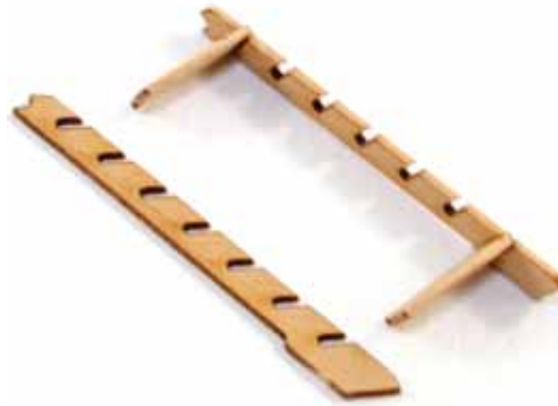
786. Glue a step into the upper and lower slot on one of the sides. When dry, glue the other side part into place.
