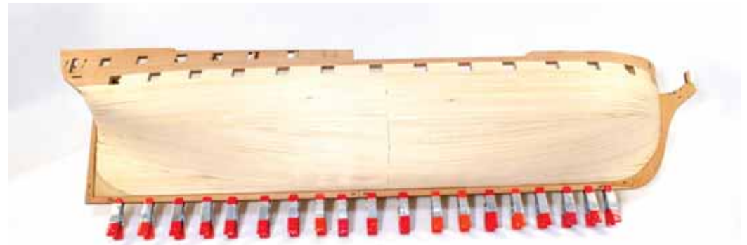
202. Now glue part #438 to the rear of the keel. Use pegs #441 to keep alignment. Clamp until dry, and then repeat the process on the opposite side of the keel with parts #439 (forward keel) and #440 (rear keel).
