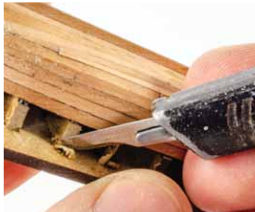
831. Slice away any protruding MDF as this will make it easier to sand the hull.
