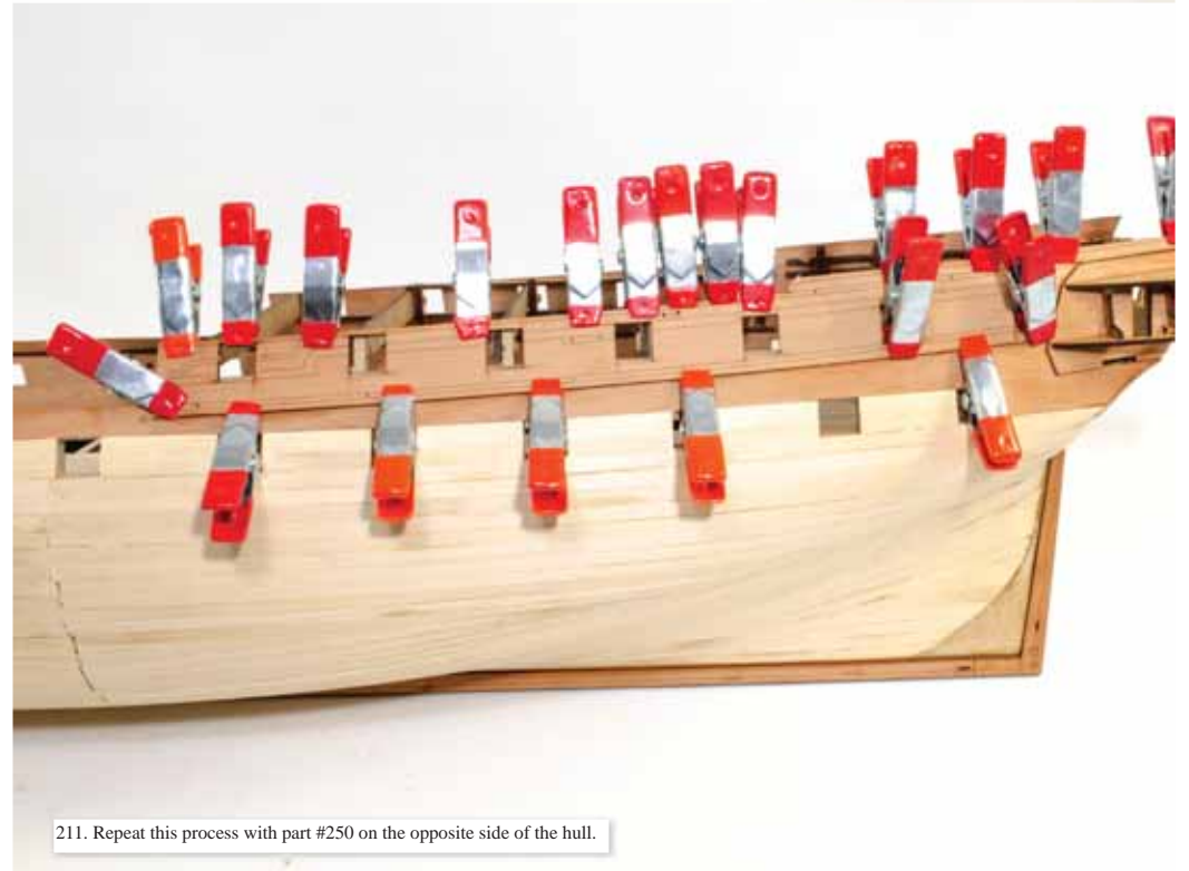
210. Glue part #246 into position on the hull, taking extreme care to ensure that everything is aligned to the quarter gallery and against the engraved line on the area below. You will see the gun ports also align. Clamp until dry.
