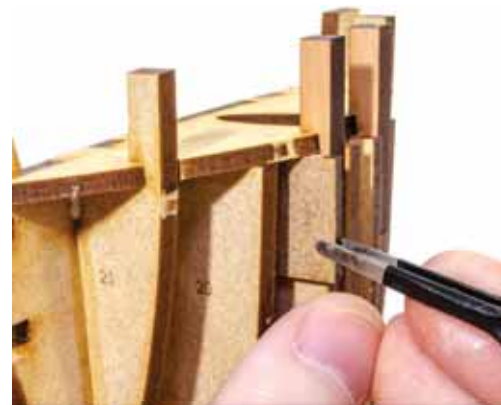
73. Glue parts #19b to the outer side of parts #19, covering the joint between the pear and MDF area.
