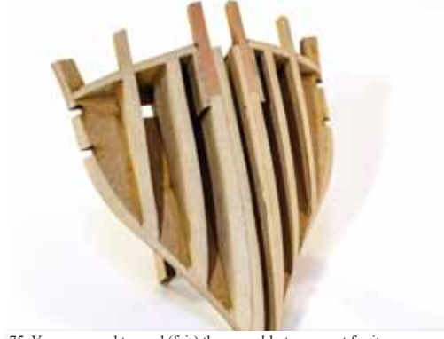
75. You now need to sand (fair) the assembly to account for its curves, as you see here. You can always under-sand this a little as it can be completed when finally fitted to the hull. Do as much as you can at this point. This photo will serve as an indication.
