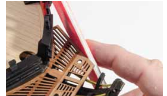
627. Take some sandpaper and sand flush any of the 'V' frames that protrude beyond the edges of the grates.
