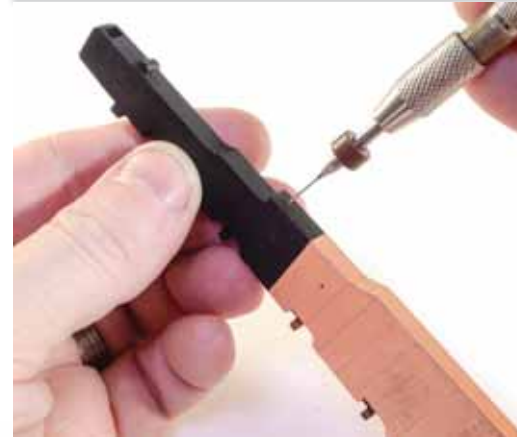
583. From the 0.6mm PE sheet, remove part PE-72. Check the position of this on your plan and drill a 1mm hole into that position in the centre of the rear of the rudder.
