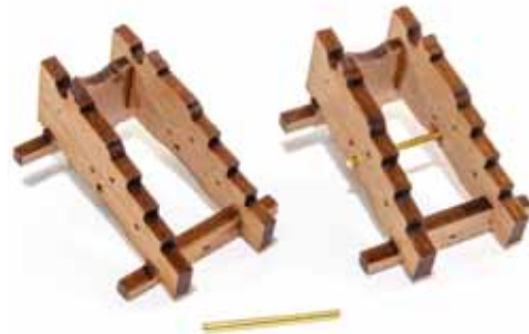
300. Cut short lengths of 0.8mm brass wire and slot through the lowermost hole on the sides of the carriage. The wire can protrude slightly on either side.
