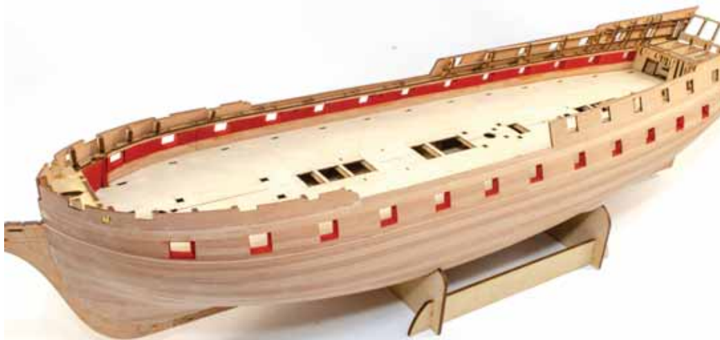
235. OPTIONAL: If you opt to use the optional laser-engraved maple deck, then you will now need this part. It's a good idea to gently smooth the deck with either 320 or 400 grade wet 'n' dry paper, followed by using a brush to remove any sanding residue from the engraved deck details.
