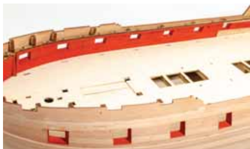
239. Varnish the exterior of the parts and then paint them in the same paint you used for the interior bulwark. Glue these into position as shown on the plan. This photo shows the forward halves in place, which are parts #260 and #266. It's important to try to align the holes in the upper ledge, with the holes in the underlying bulwark.
