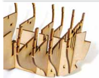
22. Glue pegs K-1 through the keel to lock bulkheads #15 and #16 permanently. You can now remove bulkhead #17 until a little later.
