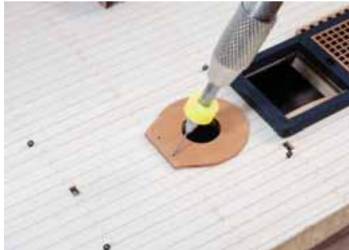
310. Glue part #278 to the deck, checking the orientation with your plan, and drill through the two holes with a 0.5mm drill.
