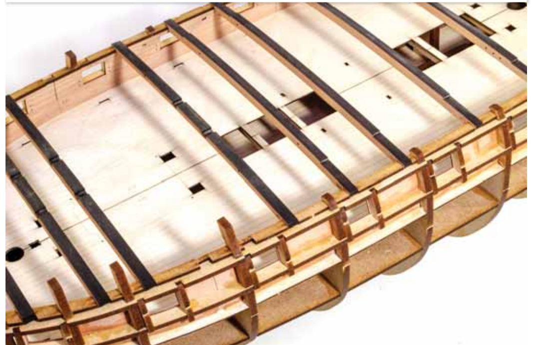
139. From the 4mm and 5mm wood sheets, remove a selection of deck beams, as well as the remaining deck beam UDI from the 4mm MDF sheet. You will notice that the strips you just fitted have the deck beam number engraved on them. Sit (NO NOT GLUE!!) the correct beam into its relative slot, from bow to stern. This is simply to gauge you have the correct positioning of the 2mm MDF strips that you recently fitted. Adjust those strips if necessary. Any adjustments should only be minor, and in terms you shouldn't really need any adjustment at all. Once you are happy that the beams sit snugly into their positions, paint some wood glue into the joint between the strips and bulkheads. NOT the deck beams themselves!
