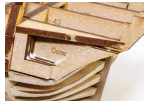
108. Glue the parts into the area seen here, directly under the last parts you fitted. This simply fills a hollow under there and gives you something solid to later work against.
