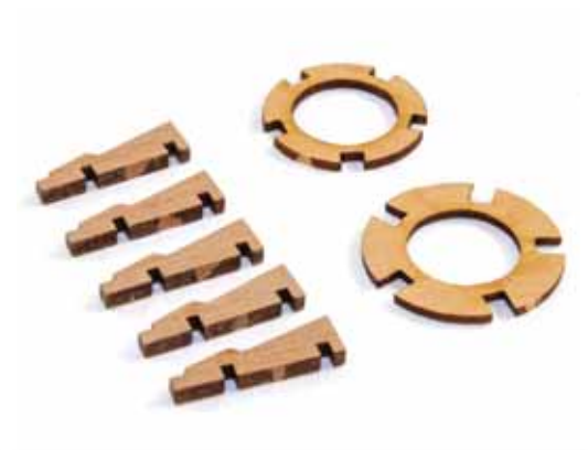
734. Indy has two capstans, and now we make the upper one. From the 2mm wood sheet, remove parts #120 from the 2mm wood sheet. From the 1mm wood sheet, remove parts #281 and #282.
