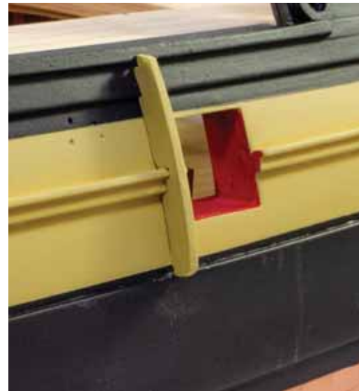
654. Again, profile these to suit your hull and the rails, then paint in yellow and glue the forward one to the hull on each side, referencing the position on your plan.
