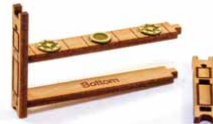
777. Glue this assembly into the middle slot on the binnacle side, noting that the scalloped end of the side part is the bottom on the binnacle. Now glue the 'Bottom' part into place in the slot adjacent to the scalloped end of the side part.
