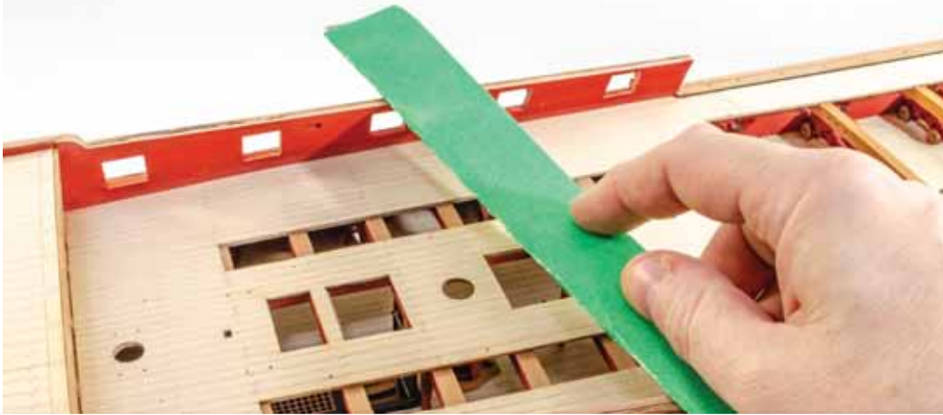
533. Here we have used a 12-inch steel rule which is covered in 110 grit sandpaper and used it to evenly sand across the top of the bulwarks, levelling them. Even though we don't show it here, PLEASE make sure all the hull openings are masked. Even out the tops of all bulwarks (poop, quarter, and fore).
