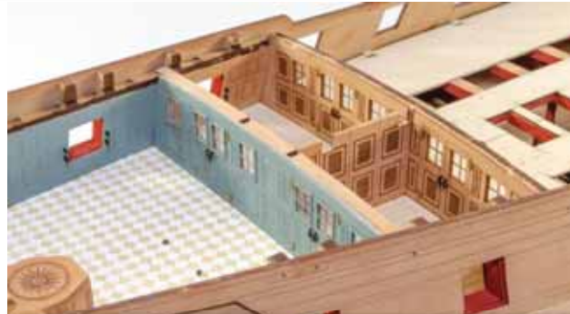
433. Take PD4 and glue into place in the numbered slot which is just in front of the rear bulkhead screen. Remove the char from the top side first. This beam, along with others in front of the rear screen, should be left in natural wood/varnish only.
