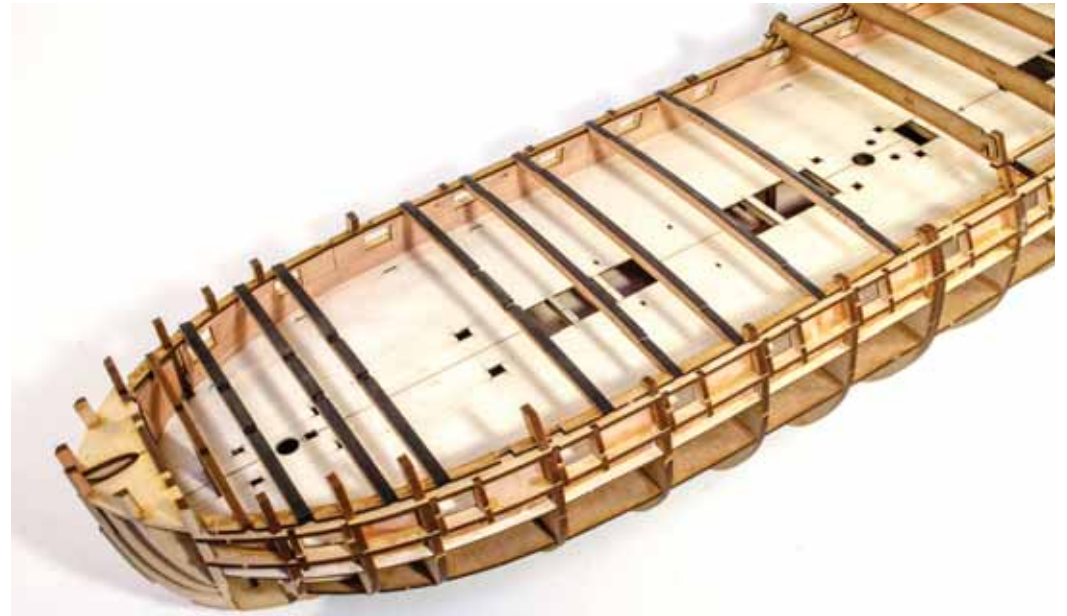
139. From the 4mm and 5mm wood sheets, remove a selection of deck beams, as well as the remaining deck beam UDI from the 4mm MDF sheet. You will notice that the strips you just fitted have the deck beam number engraved on them. Sit (NO NOT GLUE!!) the correct beam into its relative slot, from bow to stern. This is simply to gauge you have the correct positioning of the 2mm MDF strips that you recently fitted. Adjust those strips if necessary. Any adjustments should only be minor, and in terms you shouldn't really need any adjustment at all. Once you are happy that the beams sit snugly into their positions, paint some wood glue into the joint between the strips and bulkheads. NOT the deck beams themselves!
