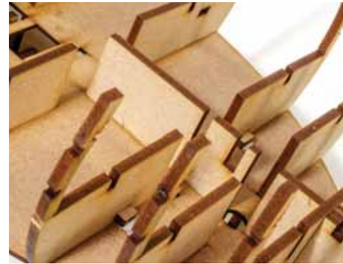
30. Carefully align this part so it sits behind bulkhead #2, and slots into bulkheads #3, #4, #5, #6, #7, #8, and #9. Do NOT glue for the moment.
