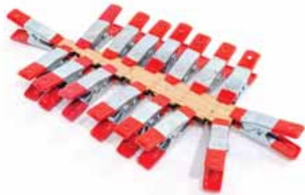
579. Glue the outer parts to the inner core. Clamp until thoroughly set.
