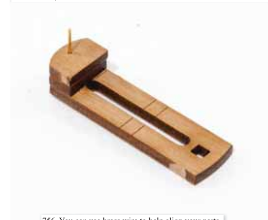
756. You can use brass wire to help align your parts.
