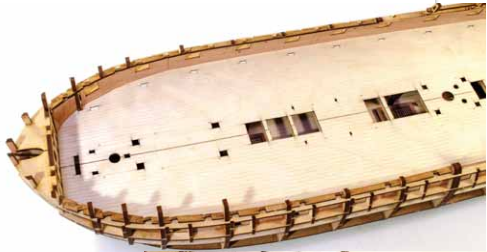
135. From the 2mm MDF sheet, remove both parts #58-F. These are the strips which will eventually hold the various deck beams.
