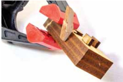
619. The jigs you have made are to help build the cathead knees. These timbers need to curve. From the 0.6mm wood sheet, remove all parts #510.
