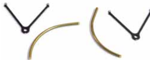
645. From the 0.4mm PE sheet, remove both parts #46. Also take the two parts of brass wire from the lanterns pack. Bend and cut the wire to the bracket profile shown on the plans.
