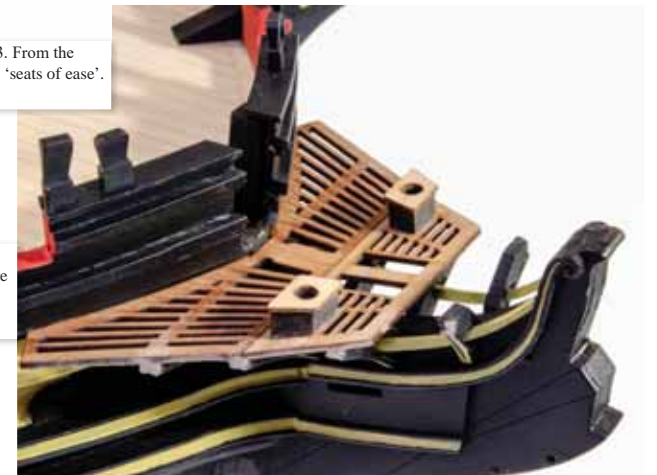
629. Glue the parts together as shown here and bevel the underside of them so that they sit horizontally onto the fore bow grate. Glue the assemblies into place. You can now paint the bow grates etc. in black.
