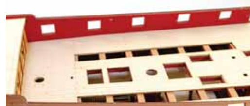
500. Paint the parts in red and fit as shown. Please remember that the position of these is slightly offset in that the inner bulwarks will be slightly higher than the area they fit to. This is to allow for the sanding angle of the ports (sills horizontal) and for them being levelled across their tops in the next stages.
