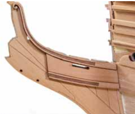
560. Trim and glue those parts to the prow as shown. Now repeat the same process with parts #215, #172, and #174 on the opposite side.
