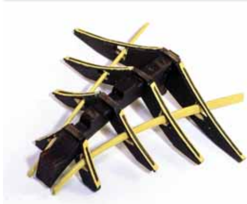
613. Slide the two narrow rails you just painted, through the bow frame assembly. You will need to slightly file/angle the openings in the frame assembly so that the rails pass through easily.
