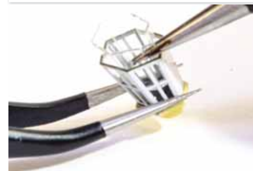
648. Remove the glazed parts from their sheet and bend into shape as shown. Push the glazing into the lantern.
