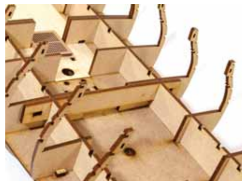
58. Slot part #11b adjacent to bulkhead #11, as shown. Glue and insert pegs through the slots as shown.
