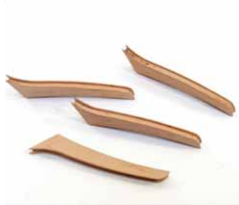
562. Sandwich the 2mm parts between the 0.6mm parts. It's an idea to round the forward edges of the 0.6mm parts first, for aesthetics.
