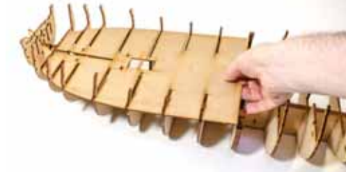
30. Carefully align this part so it sits behind bulkhead #2, and slots into bulkheads #3, #4, #5, #6, #7, #8, and #9. Do NOT glue for the moment.
