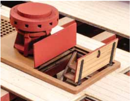
749. Glue the PE to the doors and add to eyelets PE-1 as handles. Now glue the doors into place as shown.
