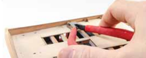
484. Use cutters to remove all the MDF bulkhead ears above deck level. Do this on all decks.
