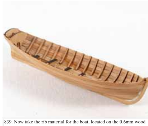
839. Now take the rib material for the boat, located on the 0.6mm wood sheet and glue them into place like this, approx. 5mm apart.
