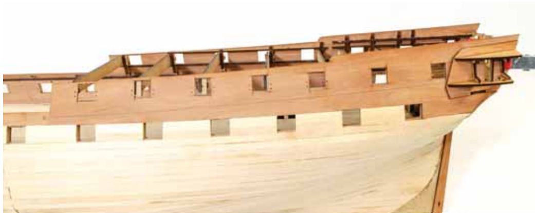
209. Before you attempt to glue these, TEMPORARILY clamp the quarter gallery skeleton assemblies into place on your hull. For the moment, these will just help with bulwark alignment and will be removed afterwards for later use.
