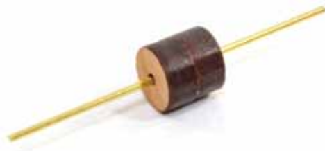
771. Glue the two thicker drum parts together using brass wire as a guide.
