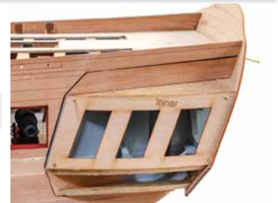
467. Test fit #518 and trim to suit your assembly. You are best making sure that the forward edge does not protrude beyond the front of the gallery. Glue/pin into place.
