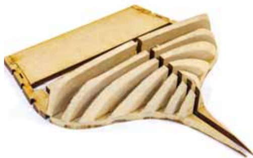
80. Sand the assembly so the curves flow into each other. You'll note the top two parts are squarer than those underneath. Please maintain that shape of those upper parts and transition that shape down to the curve of the parts below it. Final shaping can be left until the hull is faired. Sanding now simply lessens the work you need to do on a large hull.
