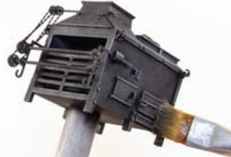
351. Firstly, prime your stove. We use Tamiya Extra Fine primer. Next, airbrush the stove in flat black, followed by a very dry brushing of a metallic pigment. We use steel pigment on the prototype. Do this for all stove parts.
