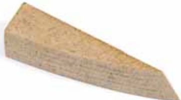
472. Remove the assembly from the model when dry and shape/sand it like this so the front of it slopes at the same angle as the engraved line on the hull. The rear side should bevel to a point flush with edge of stern.
