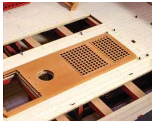
733. Glue the gratings into place. These are parts #410 and #411, found on the same 1mm wood sheet.
