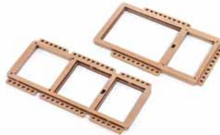
254. After char removal, the parts will look like this.
