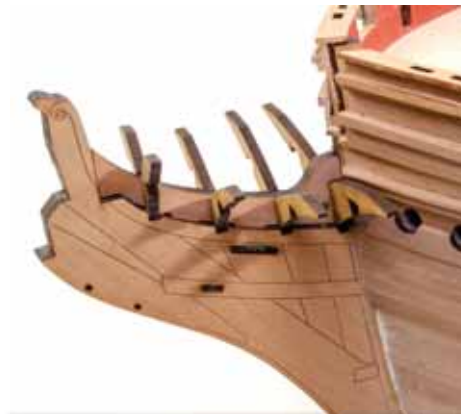
556. Before the glue dries, sit the assembly onto the hull to assure alignment. Do NOT glue into place.
